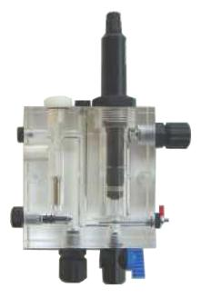
The DG7-FC is a panel-mount, ready-to-use Free Chlorine Sensor. It is designed to monitor free chlorine in drinking water, rinse water, cooling water and any other fresh water samples. The sensor provides two measurement ranges, the standard 0.05~10.00ppm, and the extended 0.01~5.00ppm for low values. The DG7-FC is compliant with EPA method 334.0 for measuring drinking water.
